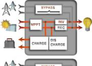
It can be running without batteries, energy shared from utility and solar to loads at the same time or alternatively. Without batteries, it can help clients to reduce the whole solar system cost and save electricity fee.
